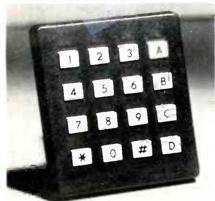
FIG. 65—A 16-KEY Touch-Tone pad similar to this one was used in the prototype to modulate an FM transmitter.
