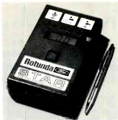
FIG. 3—SELF-TEST AUTOMATIC READOUT, or STAR, translates a diagnostic pulse string into an easily read fault code.
